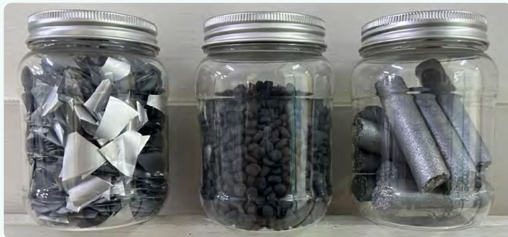
TSMC recycles discarded aluminum-plastic packaging bags (left) and reproduced them into plastic pellets (middle) and aluminum materials (right).
